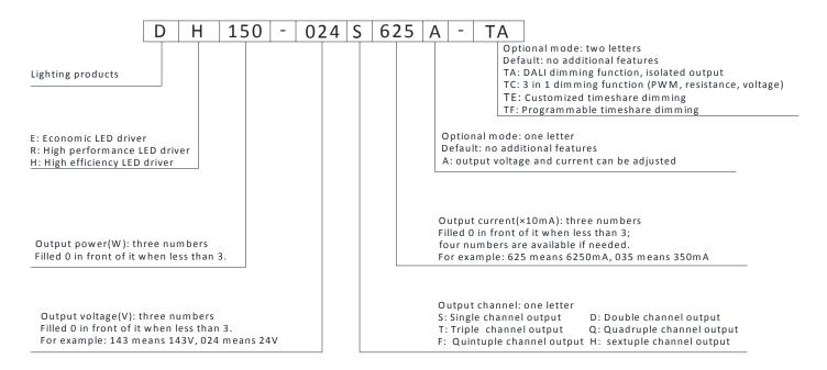
For example: DH150-024S625A-TA means: high efficiency LED driver; output power 150W; output voltage 24Vdc; output current 6250mA; single output; output voltage and current can be adjusted; with DALI dimming function and isolated output.
