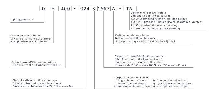
For example: DH400-024S1667A-TA means: high efficiency LED driver; output power 400W; output voltage 24Vdc; output current 16670mA; single output; output voltage and current can be adjusted; with DALI dimming function and isolated output.
