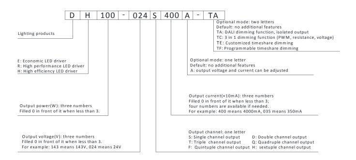
For example: DH100-024S400A-TA means: high efficiency LED driver; output power 100W; output voltage 24Vdc; output current 4000mA; single output; output voltage and current can be adjusted; with DALI dimming function and isolated output.
